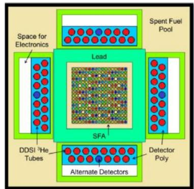
Fig. 1. Cross-sectional view of the simulated DDSI instrument.
