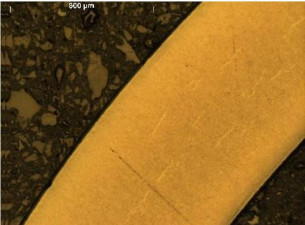
cladding waterside oxide
