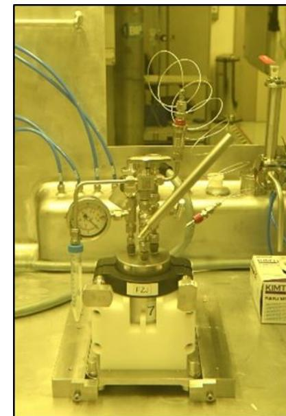
250 mL Ti-lined stainless VA steel autoclaves
