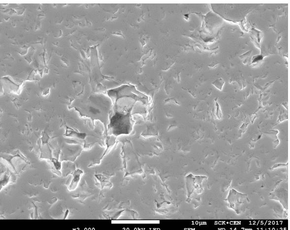
cladding waterside oxide
