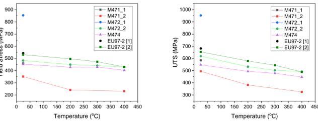
Model alloys have fully martensitic structure (except M471 standard HT). Block and lath sizes are comparable to lab-cast EUROFER. Mechanical performance was evaluated based on tensile, hardness and Charpy tests. Tensile properties of model alloys are comparable to EU97-2 whereas impact properties are superior.
